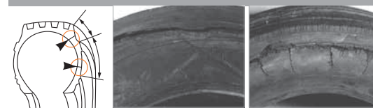
Sidewall damage due to run flat or severe under inflation
