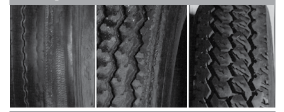
Flat spotting due to locked brakes
