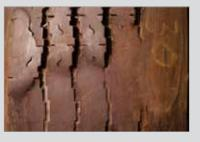
SHOULDER WEAR CAUSED BY WRONG CAMBER OR MISALIGNMENT
