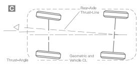
If the rear axle or wheels are toed to one side , the thrust line will not match up with the center line and the vehicle will pull—in this case—to the left.
