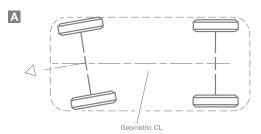
The geometric and vehicle center lines are one in the same in a properly aligned vehicle - shown in A
